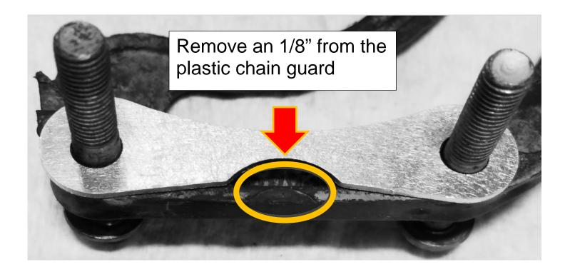
b. Next, install the Rekluse aluminum spacer between the slave cylinder housing and the plastic chain guard.
