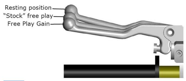
**Note:** It is very important the motor returns to idle before revving the engine again or Free Play Gain will not be correct.
