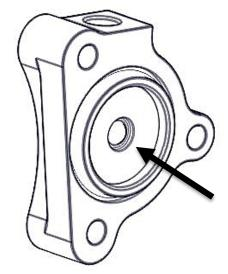
g. Repeat steps d-f until there are no air bubbles coming out in the fluid when the piston is compressed.
