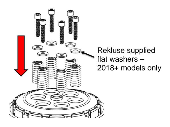
**Note:** Be sure to alternate springs, if you are using two different color springs, to keep even pressure on the clutch.
