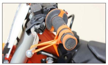
While still in **NEUTRAL**, quickly rev the engine between 5,000-7,000 RPM (1/2 to ¾ throttle), then let it return to idle. Notice the movement in the clutch lever when the engine is revved. This is your Free Play Gain.
