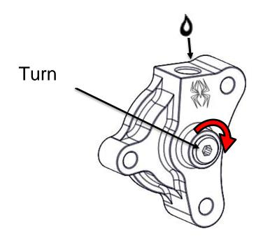
e.Use the wrench to turn the adjuster screw counterclockwise back to the initial position, with the top O-ring visible. Keep the fluid topped off as you go.
