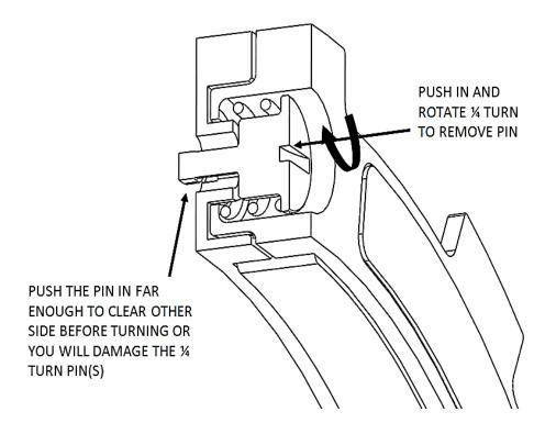
3. Remove the remaining 2 pins and springs from the same side of the EXP base.
