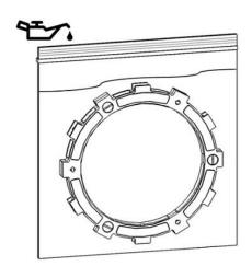
2. Install all the Rekluse basket sleeves into the basket slots. Make sure the bottom of the sleeve is facing down, and the sleeve tabs sit against the inside of the basket. See pictures for reference.
