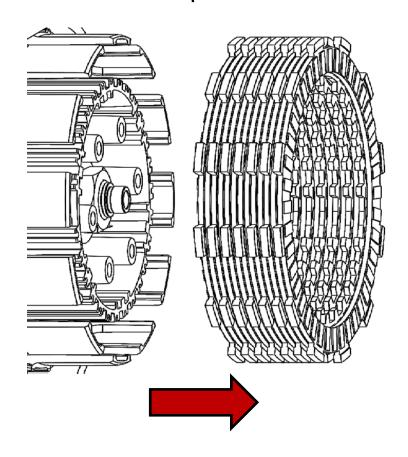
6. Inspect the clutch basket for spring damper play or notching. **Do not install sleeves or use product with a notched basket.** Notched basket tang faces or worn dampers can cause the sleeves to break. Do not use baskets that have been filed, machined, or modified on the tangs. Replace basket if necessary.
