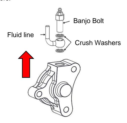
d. Attach the clutch fluid line to the Rekluse slave cylinder using the OE banjo bolt and the 2 new crush washers from Rekluse. *Make sure the clutch fluid line is between the 2 crush washers*.
